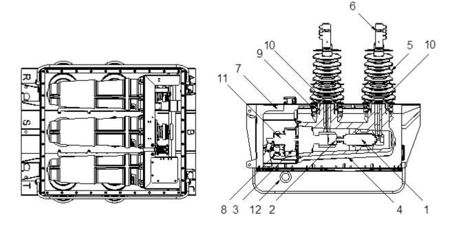
Note: Current Transformer position varies in OSM 30x and OSM 31x series reclosers. OSM 300 model shown.
