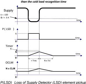
Cold Load Pickup when Loss of Supply is shorter
