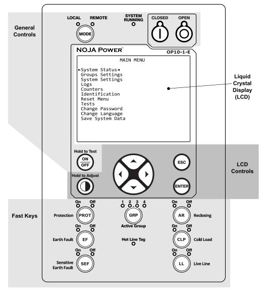
The layout of the Panel is illustrated above, each of the pushbutton groups are explained in the following sections.
