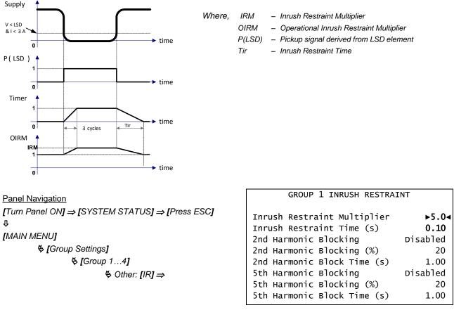
Operation of the Inrush element is illustrated in the diagram below.
