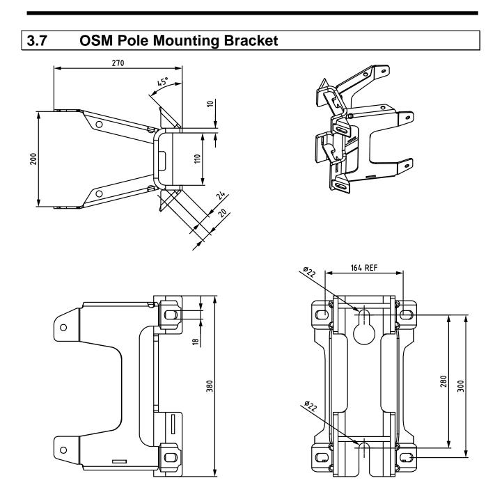
**Note:** The standard bracket shipped, unless specified otherwise, allows for the use of C-clamp mounting as an alternative to through bolt mounting.
