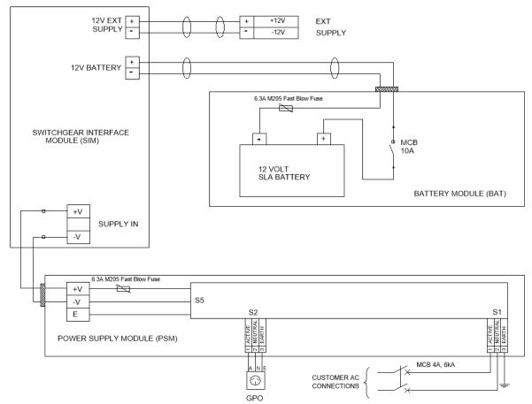
Power Supply Wiring Diagram
