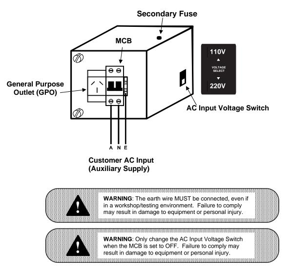
**Note:** The Dual Input PSM module includes two Customer AC Input connections, two AC Input Voltage Switches and two Secondary Fuses. Please refer to Section 10.5 Spare Parts List .
