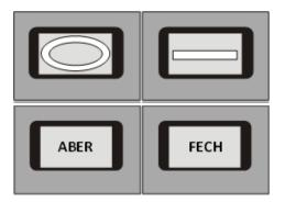
The OSM position indicator is located under a protective cover underneath the tank and is clearly visible from the ground.
