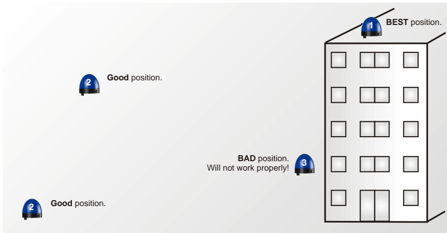
Figure 4-1: Suitable places of installation for the CMGPS 588
