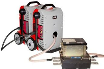
This makes it easier to pass the cable through the hole of each unit and allows the infrared communications channel of the Raptor units to work correctly (this communication, in both sides of units, is designed for being viewed directly and at a distance of less than 1 meter).
