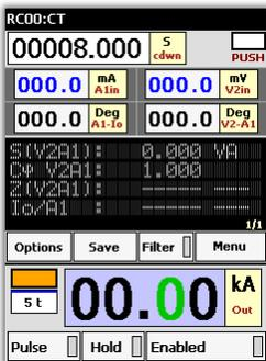
Template designed to verify the transformation ratio in current measurement and/or current protection transformers (CT).
