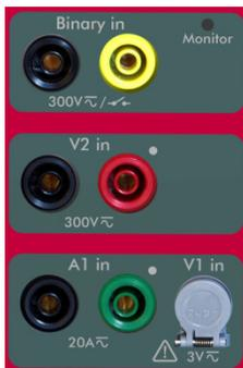
In addition to the binary input related to the chronometer, the main panel of the Raptor-MS unit has three measurement inputs, two for voltage and one for current.
