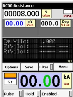
The contact resistance of circuit breaker poles, sectionalizers, busbar connection points, and cables, etc. must be verified during any start-up or maintenance of primary equipment. This resistance is characterised by its low value, around tenths of micro-ohms. The only way to measure them is via the 4-wire measurement, which consists of injecting a current of sufficient value so as to generate sufficient voltage drop to be measured with certain accuracy.
