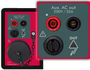
The Raptor-MS unit has auxiliary outputs to be able to inject small currents or high voltages that are essential in certain tests.
