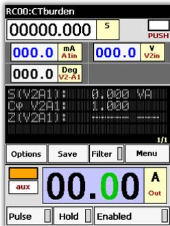
This template enables us to determine, very accurately, the burden that is connected in the secondary of a CT. Accurate knowledge of this value as well as of its power factor is very important to determine if the CT is suitable or not for this burden. This information must be used together with the nominal power of the CT and its magnetisation curve.
