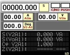
The controls that show the measurements taken by the equipment are located here. They can be *hardware* measurements (direct readings made by the Raptor-MS) or *calculated* measurements (processed based on *hardware* meters). You can modify the meters you want to be displayed
