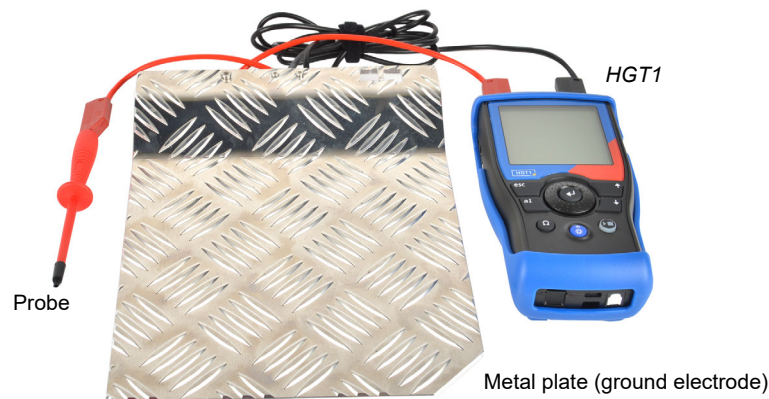
Figure 8-13: HGT1 hardware setup according to EN 50522
