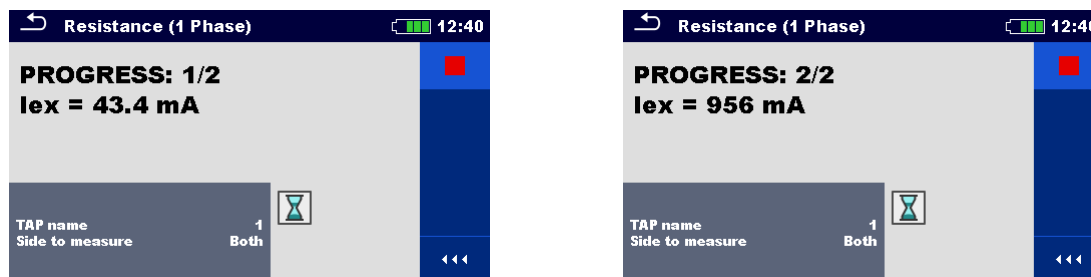
Figure 11.17: Progress indicator at single-phase transformer winding resistance measurement: H side testing in progress (left), X side testing in progress (left)
