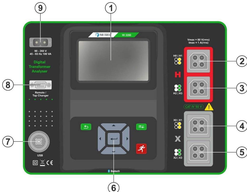
Figure 4.1: The operator's panel
