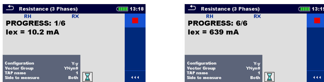
Figure 11.21: Progress indicator at three-phase transformer winding resistance measurement: first (1/6) test in progress (left) and last (6/6) test in progress (right)
