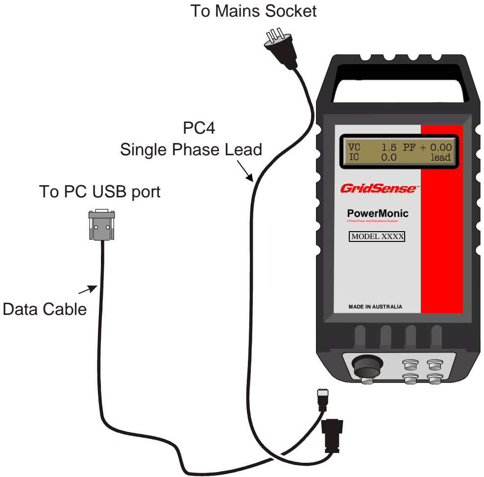
Fig 16 – Connecting the PowerMonic to the PC
